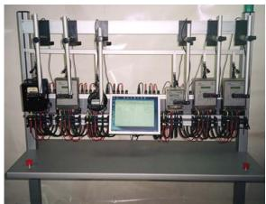
The unit is intended for calibration of electronic and inductive single- and three-phase meters of active and reactive energy. It allows to automatically calibrate 6, 12 or 24 meters.
