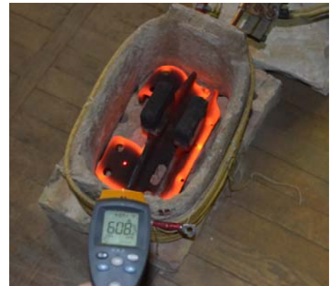
Heating of the cast-iron brake shoe of subway car reducer
