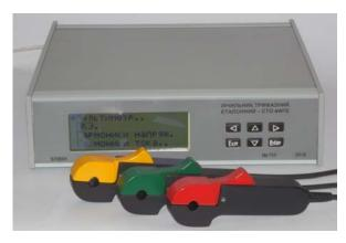
The standard is intended for checking electronic and inductive single- and three-phase meters of active and reactive energy, as well as the means for controlling the parameters of electric power quality. Depending on the performance, it allows to automatically detect an error of the meters and power quality analyzers that are checked, and control the parameters of input signals.
