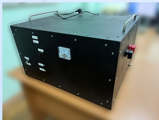
Standardized microsecond pulse interference simulator (CWG 1.2/50–8/20 μs)
