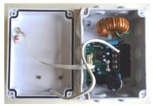
The converter is intended to convert constant (alternating) voltage of the network, renewable energy sources (RES) or batteries of 35 ... 380V into a constant voltage of 350 ... 405V. It can be connected to a stand-alone (grid) inverter or to charge batteries.
